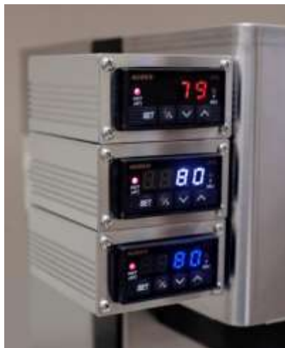
Рисунок 2.3 – PID Retrofit KIT for Rancilio Silvia /w pre-infusion
